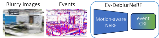
Figure 1. Ev-DeblurNeRF combines blurry images and events to recover sharp radiance fields. A motion-aware NeRF recovers motion and a learnable event camera response function models real camera’s non-idealities, enabling high-quality reconstructions.
