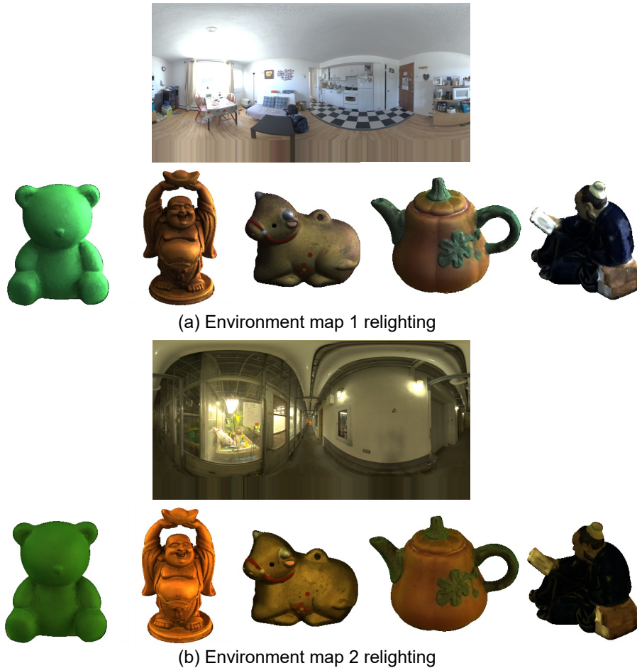
Figure S13. Environment map rendering. We render various objects with two environment maps. Both of rendering results show faithful relighting by reconstructed surface normals, spatially varying BRDFs, and visibility.
